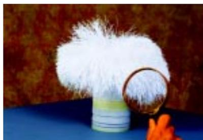
*A single membrane module which has been cut open to show its 10,000 fibers. FPW will have a total of 4,500 membrane modules once the plant expansion is complete..*
