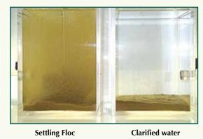
The floc-laden water enters sedimentation basins where the majority of the solids settle. Specially designed inclined settling plates affixed in each basin are vital to achieving proper settling. Water exiting the sedimentation basins is called clarified water.
