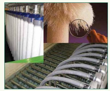
Clockwise: module rack, cut fibers, submerged membranes
