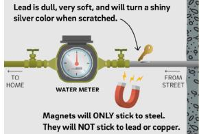
**Step 2:** With some sandpaper or emery cloth, clean a small portion of the pipe that is easy to reach anywhere between the water meter and the outside wall. Once the pipe is clean and silver in color, move onto step 3. If the pipe color is penny-colored, you have a copper service and do not need to continue onto the rest of the test.
