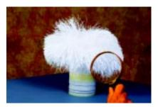
A single membrane module which has been cut open to show its 10,000 fibers. FPW will have a total of 4,500 membrane modules once the plant expansion is complete ..
